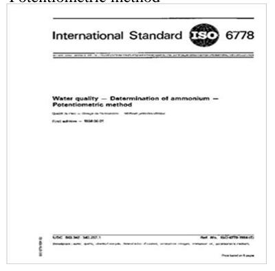
Specifies a procedure using an ammonia-sensing membrane probe for raw and waste water and sewage. The procedure is applicable to ammonium nitrogen concentration of up to 50 mg/l. The limit of detection is defined as the limit of Nernstian response under the conditions specified and has a value corresponding to approximately 0,2 mg/l. This title may contain less than 24 pages of technical content.
